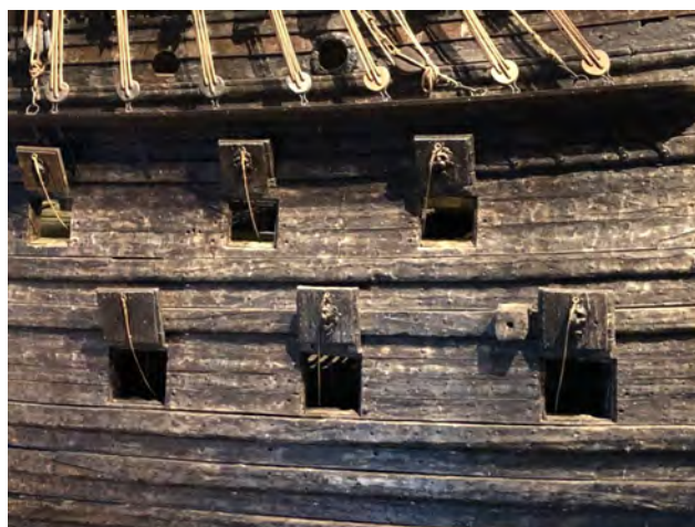
The ship was the first in the Swedish Navy to have two gun decks.
